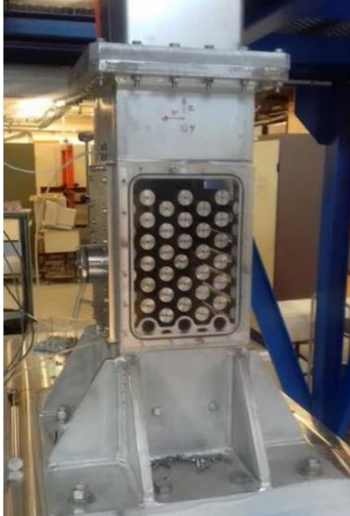
Figure 12. TITAN test section consisting of a tube array with a tringle lattice exposed to a two-phase cross-flow. This CEA experiment is performed at high flow velocities and also deals with fluid-elastic instability phenomenon.
