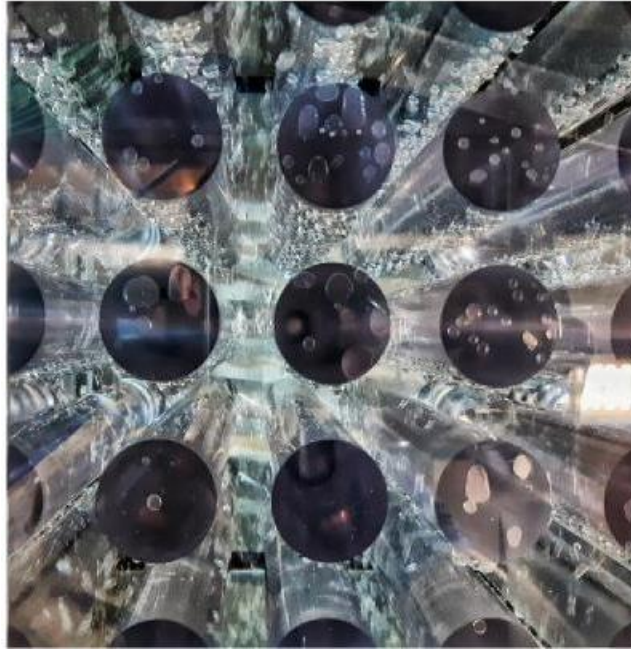
Figure 11. TREFLE test section with 5x5 tube array, exposed to a two-phase cross-flow at IRSN. The tubes are arranged in a square lattice, two of these vibrate, while the rest are rigid.
