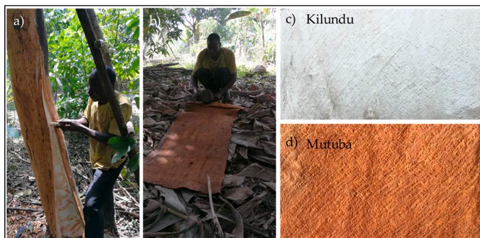
Fig. 2. a) Bark’s manual extraction; b) pummeling process with a wooden beater; c) detail of the different samples with their name.
