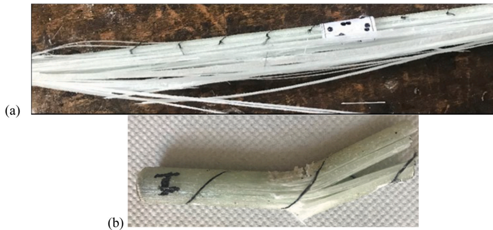
Fig. 7. Representative failure modes of NPC GFRP Rebars in (a) Tensile and (b) Short-Beam Tests.
