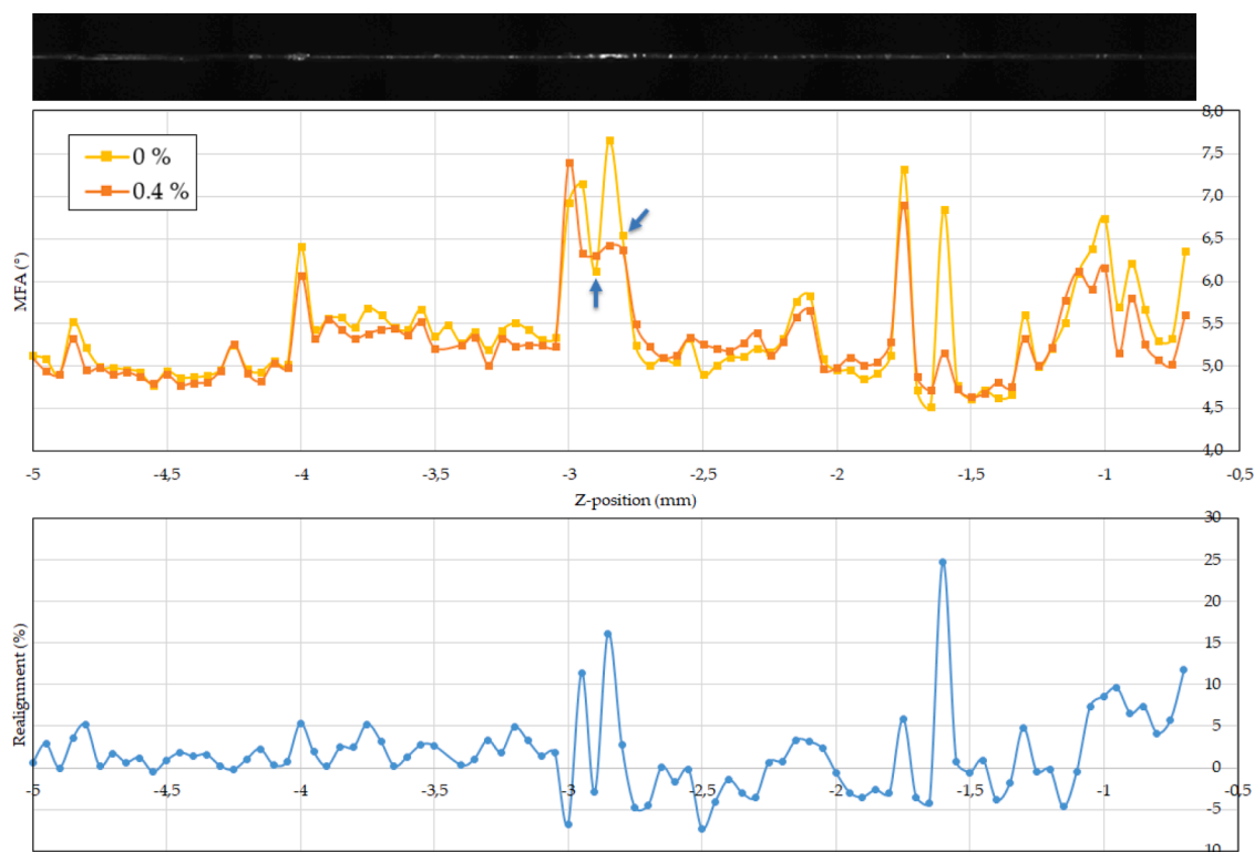
Fig. 11. View of fibre B_2 under polarized light revealing defects as bright areas (top); MFA measurements along the fibre at different strains (from 0 to 0.4%) using setting 3 (middle); and corresponding realignment calculated between the first and last tensile steps (bottom). The arrows point out values where a misalignment of the fibre thanks to the vertical axis might induce error in the resulting MFA.
