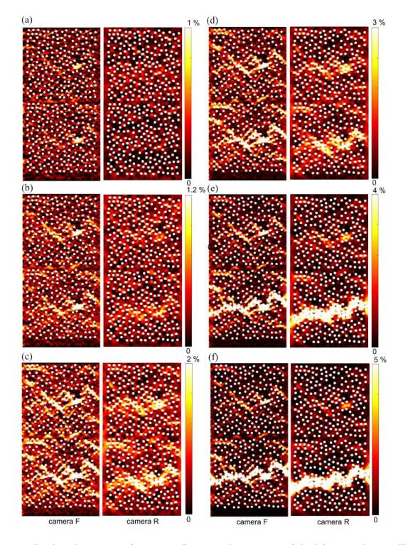
Figure 8: Local axial strain maps for specimen D20-w1 at discrete points of the deformation history. The macroscopic longitudinal strain  $\langle E_{yy} \rangle$  is equal to (a) 0.16%, (b) 0.27%, (c) 0.65%, (d) 0.77%, (e) 1% and (f) 1.2%. These levels are depicted with dotted lines in Figure 4(b). The strain fields were computed by means of FE-based DIC using images collected simultaneously by both cameras.
