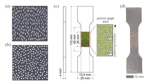
Figure 1: (a,b) Random porous architectures explored in this study. They are generated by means a numerical algorithm, and contain random distributions of equisized (a) elliptical and (b) circular pores at 20% volume fraction. The elliptical pores have identical orientation and constant aspect ratio w = 0.3. (c) Geometry of the tensile dogbone specimen comprising two identical porous cells. (d) Optical front-view of the *as-manufactured* tensile specimen.
