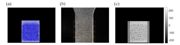
Figure 13: (a) Gmsh generated mesh to be backtracked and superimposed onto the nominal mask. (b) Reference image of Camera F for specimen D20-w03 with the coarse backtracking mesh depicted in orange. (c) Gray level residual map to backtrack the mesh of specimen D20-w03 and Camera F showing that the backtracking procedure was successful.
