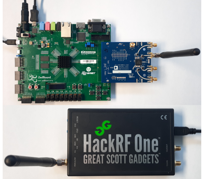
Fig. 13: Laboratory test bench: HackRF SDR sends a traffic of preambles - AD9361 RF front-end receives an RF signal and downgrades the signal to baseband - Our program runs on ARM Cortex-A9 (Xilinx Zynq 7020 SoC) and processes received signal in real-time to detect preambles.
