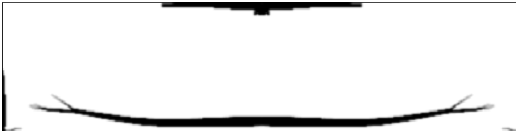
(c) Optimized layout with q = 3 , 200 design iterations with p_E = 3, p_\alpha = 3, p_{\sigma_y} = 3 and filter radius r = 0.015 .
