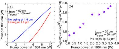
Figure 2: (a) Simulation of the output power from the amplifier at 808 nm as a function of the pump power at 1064 nm for a 60 cm-long Tm:ZBLAN fiber; (b) a preliminary gain measurement at 808 nm.
