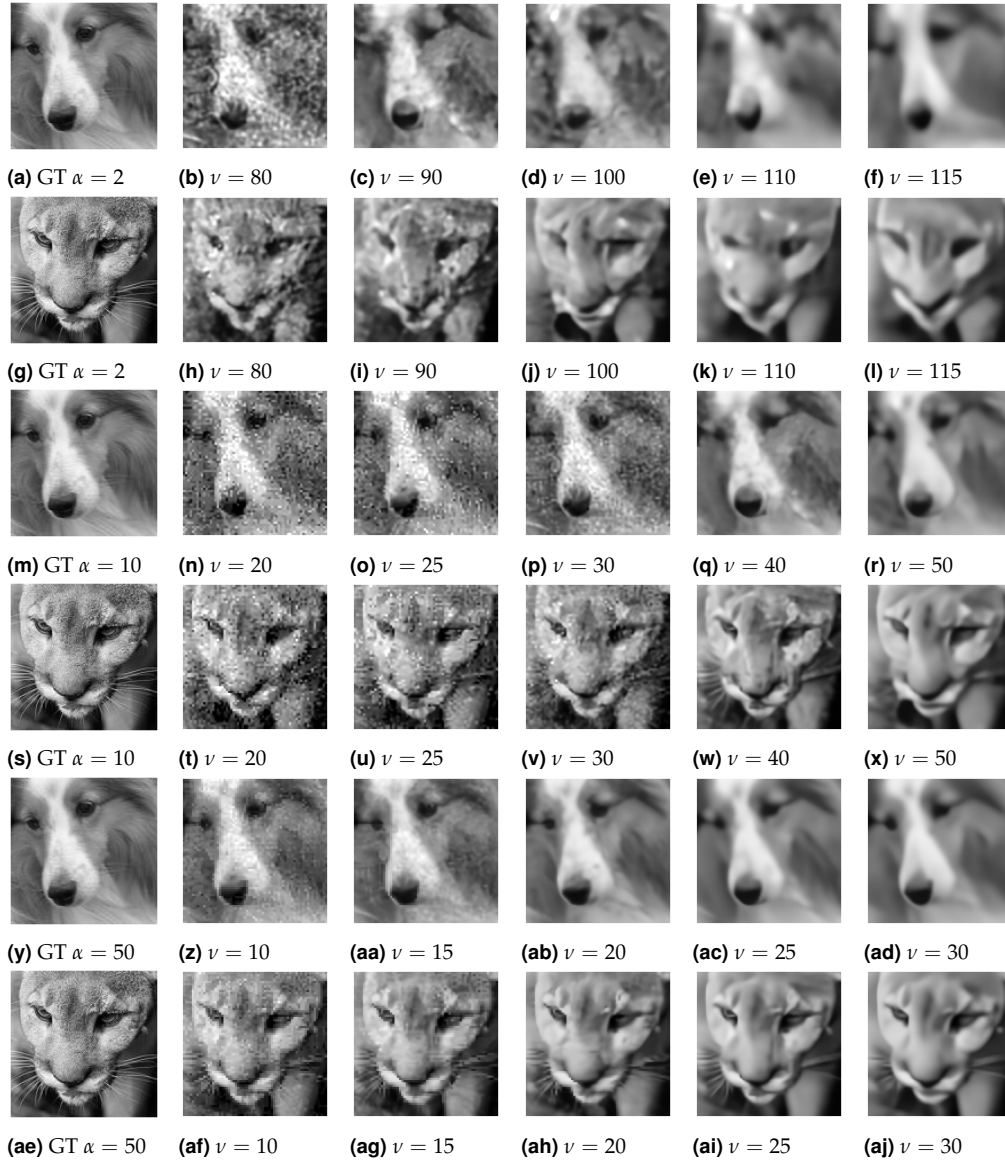
Fig. S1. Images reconstructed by Pinv-PnP for different noise levels \nu and image intensities \alpha . From top to bottom, we consider \alpha = 2, 10 , and 50 photons. The simulations consider the square subsampling strategy with \times 4 reduction for 128 \times 128 images.
