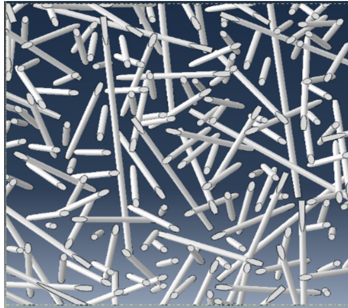
Figure 1. 2D visualization of fibers randomly oriented in space.
