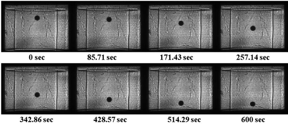
**Figure 22.** X-ray radiographic images of a sulfur sample during the fall of a Pt sphere at 0.25 GPa and 420 K, as recorded by a PCO Edge camera. The sample/diamond, sample/NaCl and diamond/hBN interfaces can be observed.
