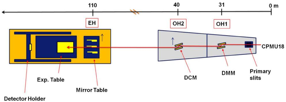
**Figure 3.** Schematic of the simplified optical configuration of the beamline ID27 (top view). CPMU18: Cryogenic Permanent Magnet Undulator (18 mm magnetic period); DMM: Double-multilayer Mirrors; DCM: Double-Crystal Monochromator. The blue arrow in OH2 indicates the horizontal movement of the DCM that enables ‘pink’ beam operation.
