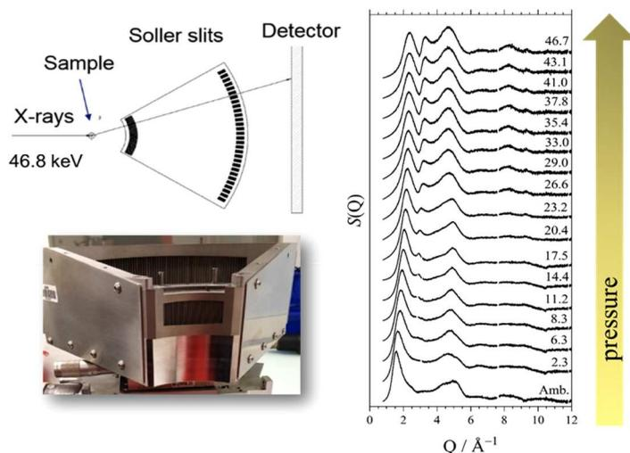
**Figure 25.** Left: Photograph of ID27 Soller slit system and its basic principle. Pressure evolution of the  $\text{SiO}_2$  glass structure factor measured in monochromatic mode up to 46.7 GPa. Exposure time: 90 s.
