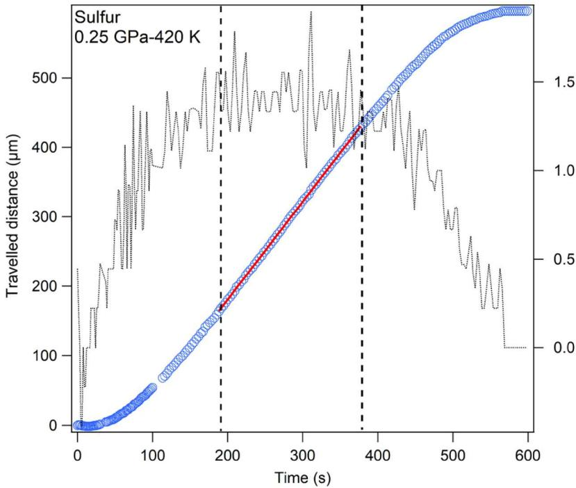
**Figure 23.** Travelled distance vs. time for the Pt sphere falling in liquid sulfur at 0.25 GPa–420 K and shown in Figure 22. Symbols in blue are experimental data. The black dotted line shows the numerical derivative of the data. The vertical lines delimit the region where the velocity of the sphere is maximal and constant. The red line is a fit of the distance-time plot in this region.
