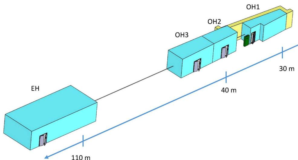
**Figure 1.** Overall layout of the ID27 beamline. The indicated lengths are the distances between the centre of the straight section of the undulators and the centre of the hatch. OH: Optical Hatch, EH: Experimental Hatch.
