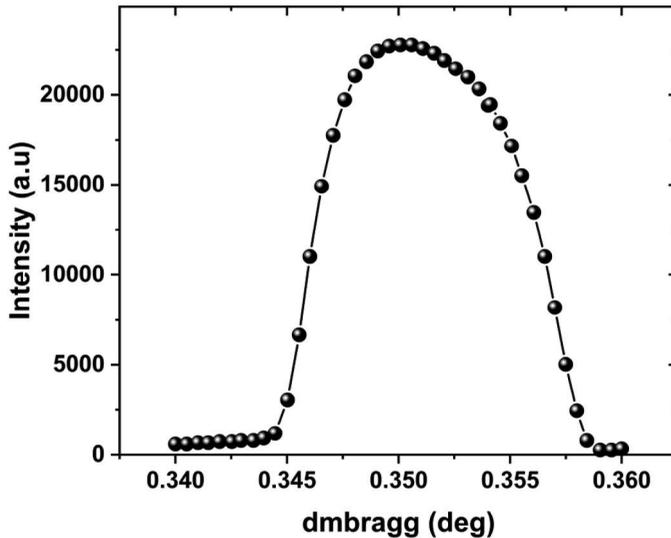
**Figure 5.** Reflectivity curve of ID27 double-multilayer mirrors.
