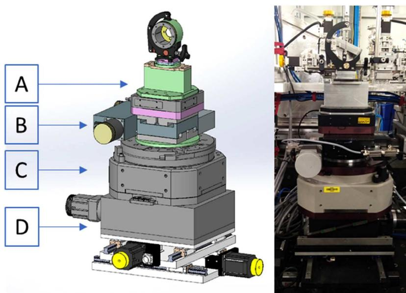
**Figure 11.** Schematic and photograph of ID27 nano-goniometer for diamond anvil cells. (A) DAC holder and XYZ piezo-stage. (B) XY micro-translation stage. (C) LabMotion aerodynamic rotation. (D) XYZ micro-translation stage.
