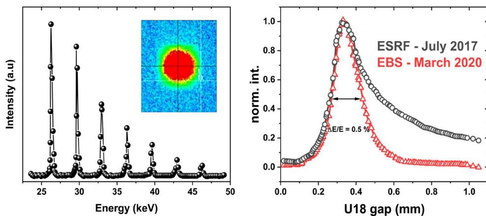
**Figure 24.** Left: ID27 undulator harmonics after the silicon (111) double-crystal monochromator. Insert image: 'pink' beam observed using an X-ray beam viewer located at 45 m from the EBS X-ray source. Right: Comparison of the shape and width of an undulator harmonic before and after EBS (courtesy of M. Burghammer, ID13, ESRF).
