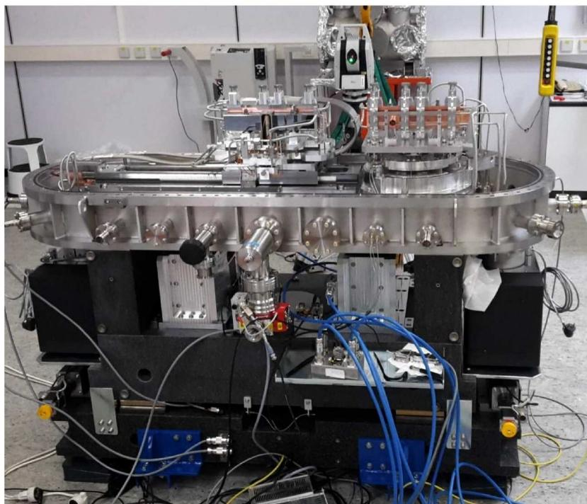
**Figure 4.** Schematic (top) and photograph (bottom) of ID27 fixed-exit double-multilayer mirror system. 1: First mirror; 2: Second mirror; 3: First mirror mechanics (Pitch); 4: Translation of second mirror along the X-ray beam; 5 and 6: Translations normal to the X-ray beam for Bragg angle and position adjustments. The black arrows indicate the vertical translation hidden inside the granite structure.
