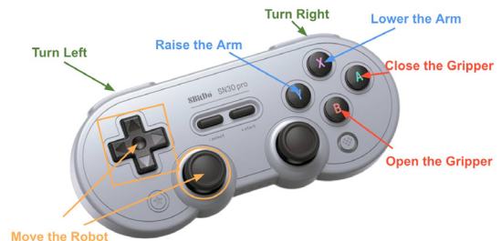
Figure 2. Interface to help getting started with the manual control of the robots
