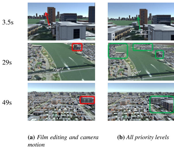
Figure 8: Ablation study: viewpoints quality. (a) Considering film editing and camera motion costs is not sufficient: (top) the motion space is not ensured, (middle and bottom) the context is badly conveyed. (b) Considering viewpoint quality costs enables to (top) better enforce the motion space and to (middle) better convey the context, among which (bottom) the landing skyport.
