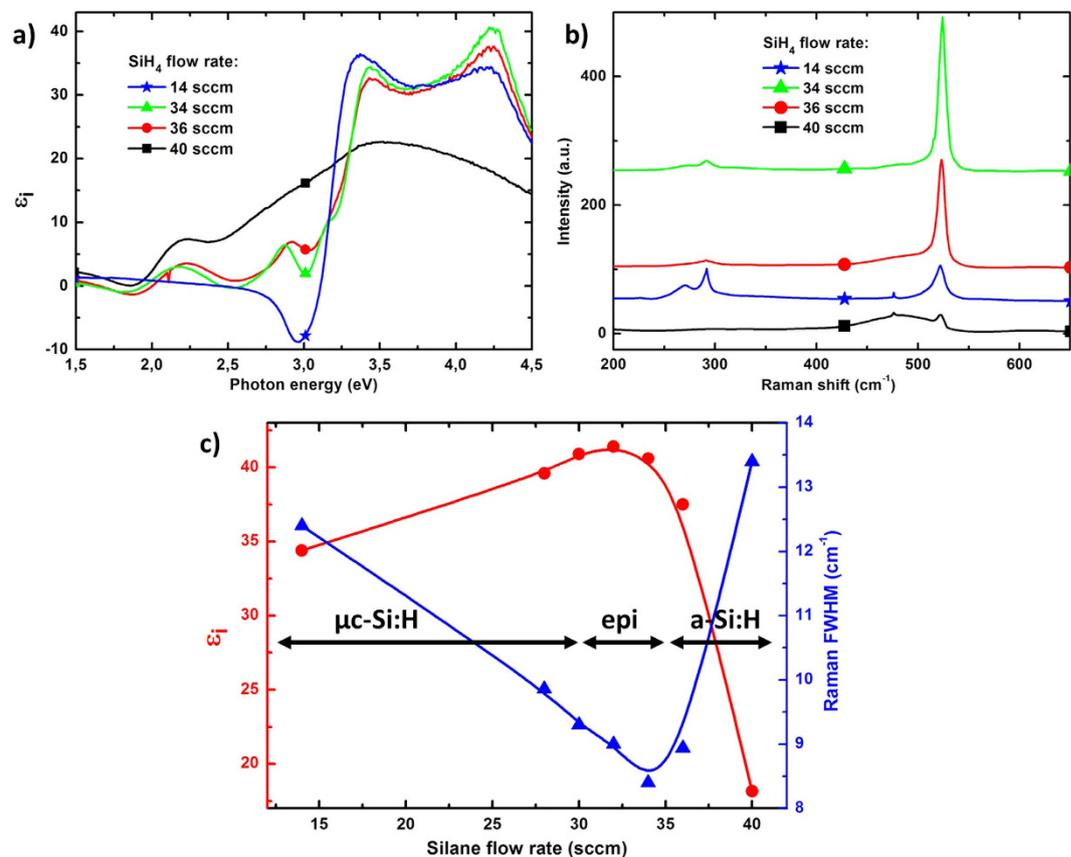
**Figure 2.** (a) Pseudo-dielectric function  $\epsilon_i$  of PECVD silicon layers deposited from  $\text{SiH}_4/\text{H}_2$  on plasma cleaned GaAs wafers with various silane flow rate: 14 sccm (stars), 34 sccm (triangles), 36 sccm (circles) and 40 sccm (squares). (b) Corresponding Raman spectra. (c) Left  $\epsilon_i$  at 4.2 eV (circles) as a function of the silane flow rate. Right: FWHM of the Raman c-Si peak FWHM as a function of silane flow rate (triangles).
