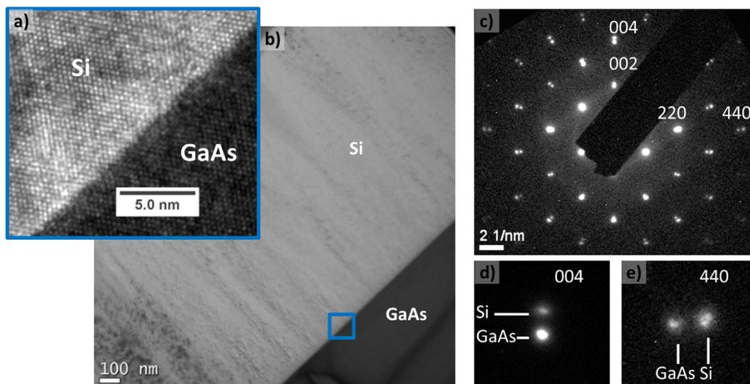
**Figure 5.** (a) HRTEM image along [110] axis of epi-Si/GaAs interface. (b) Low magnification cross section picture of a 650 nm thick epi-Si layer on GaAs. (c) Diffraction pattern of PECVD epi-Si/GaAs interface: the double points visible for each reflection (e.g. see zooms (d,e)) are the signature of both Si and GaAs lattices.
