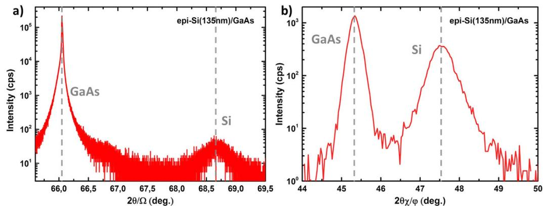
**Figure 6.** (a) High resolution XRD measurement of reflection from the PECVD (004) planes parallel to the surface of the epi-Si film on (001)-oriented GaAs. (b) Grazing incidence XRD measurement of reflections from the {220} planes perpendicular to the surface, measured on the same sample.
