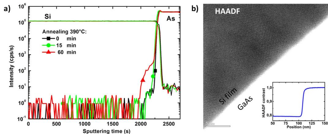
**Figure 4.** (a) SIMS profiles of Si and As across the PECVD epi-Si (1450 nm)/GaAs interface. The profiles are measured for the same sample before (squares) and after annealing at 390 °C in air for 15 min (circles) and 60 min (triangles). (b) STEM HAADF image of the interface with the inset showing intensity profile across the epi-Si/GaAs interface.
