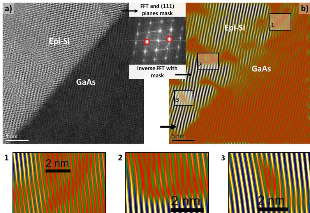
**Figure 3.** (a) High resolution STEM cross section along<sup>1-10</sup> axis of PECVD epi-Si/GaAs interface. A mask is applied to the Fourier transformed image for selecting (111) planes, and the TEM image (b) is reconstructed by inverse FFT algorithm keeping only the contribution of (111) planes. 1, 2 and 3 are zoom on crystal defects.
