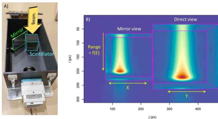
**Figure 1.** A) SCICOPRO setup consisting of a  $10 \times 10 \times 10 \text{ cm}^3$  BC-412 plastic scintillator, a mirror oriented at  $45^\circ$  to the cube and a fast camera. B) The images recorded by the camera consist of a direct projection and a mirror-reflected projection of the scintillation distribution produced by each pulse in the scintillator.
