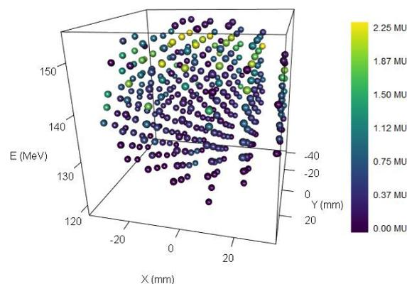
**Figure 2.** PBs characteristics measured with SCICOPRO for the irradiation plan producing a uniform dose distribution of 0.8 Gy in a 5 cm diameter sphere. Each PB is represented spatially by its X and Y positions and energy (vertical axis). The PB intensity is represented by the colour scale. For clarity, only the measured characteristics are shown here as they closely match the planned characteristics.
