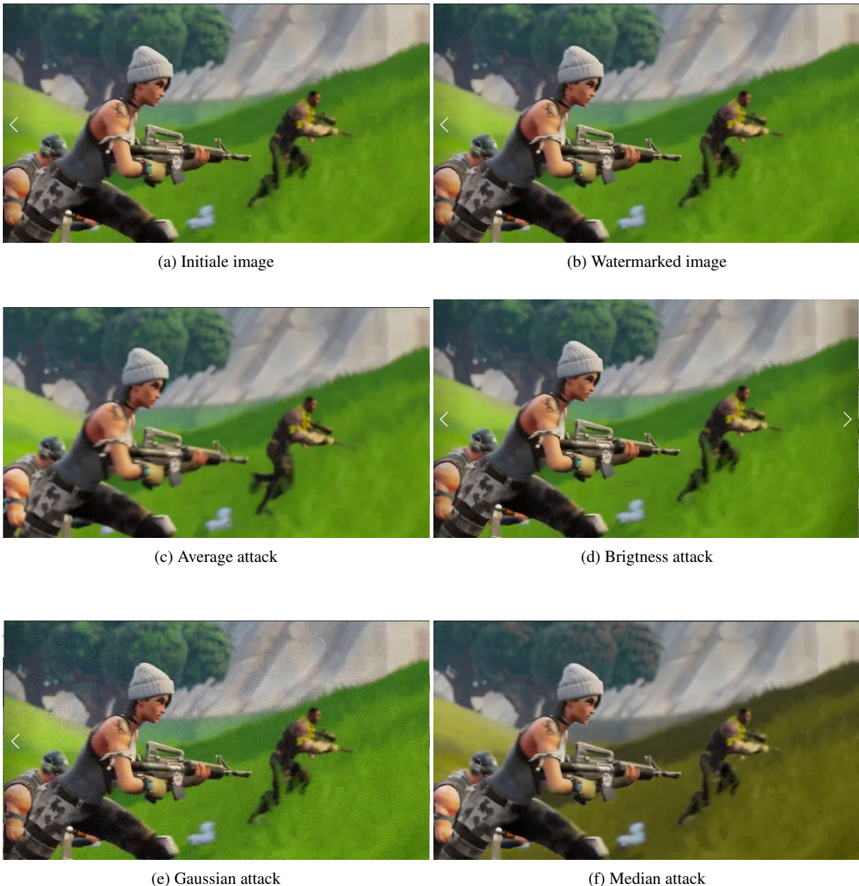
Figure 7: Same attacks:a) Initial image, b) Watermarked image, c) Average filtering 5, d) Brightness, e) Gaussian noise (0.05), f) Median filtering 9x9.
