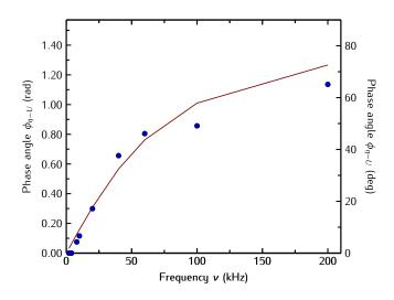
Figure 4. Phase angle  $\phi_{\eta-U}$  between the driving voltage U(t) and the strain  $\eta(t)$  as function of frequency  $\nu$ . The filled symbols are extracted from the experimental data and the solid line is the result from the fit using Equation 4 with  $\gamma = 0.5 \text{ GHz}$  to the experimental data.
