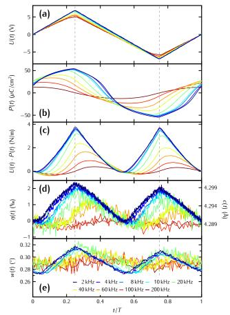
Figure 3. **a)** Applied sawtooth voltage U(t/T) normalized to by the period T of the frequency. **b)** Measured polarization P(t/T) of the FE as obtained by the integraton of the switching current over time. **c)** Product  $U(t/T) \times P(t/T)$  that closely resembles the time-response of the measured transient strain  $\eta(t/T)$  of the FE shown in panel d). **e)** Peak width change w(t/T) of the PZT Bragg reflection.
