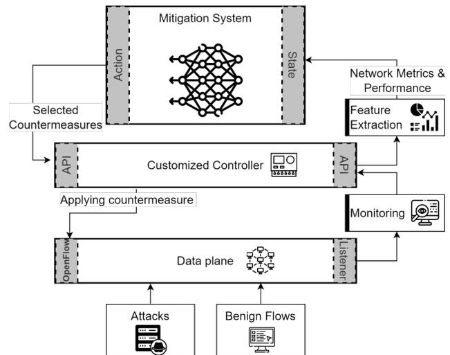
Fig. 4. System Architecture.
