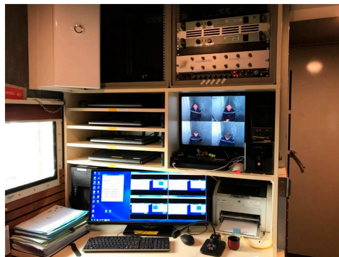
Figure 3. Interior view of the mobile hearing laboratory. In the center right of the setup, a video screen displays images of participants situated in the four booths. Positioned in the center left are four portable “follower” computers equipped with fold-down screens, to which the screens, keyboards, and mice of each booth are connected. Beneath these computers, there is the “leader” computer, positioned at the bottom center, with its screen visible. Additionally, the screens corresponding to the “follower” computers are also visible.
