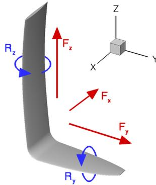
Figure 10: Sign conventions for forces and rotations of the L-foil. The hydrofoil advances in the positive  $X$ -direction. Figure not to scale.
