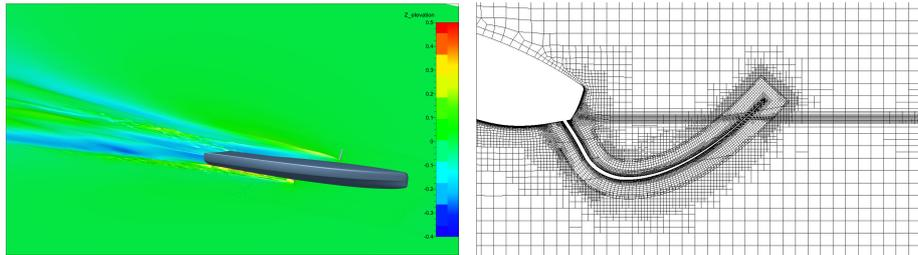
Figure 27: Simulation of a full yacht hull with hydrofoils.
