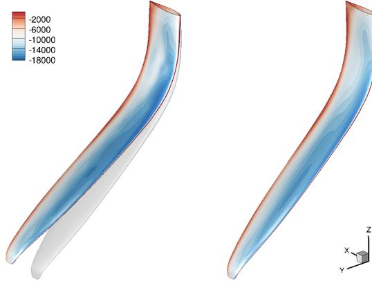
Figure 25: Comparison of foil shapes and suction-side pressure for the deformed (left) and rigid (right) Nacra 17 hydrofoil.
