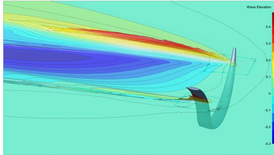
Figure 19: Wave field around the IMOCA foil.
