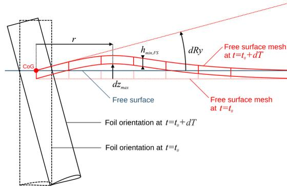
Figure 7: Analytical weighted deformation: the effect of a quasi-static pitch rotation on the free-surface mesh.
