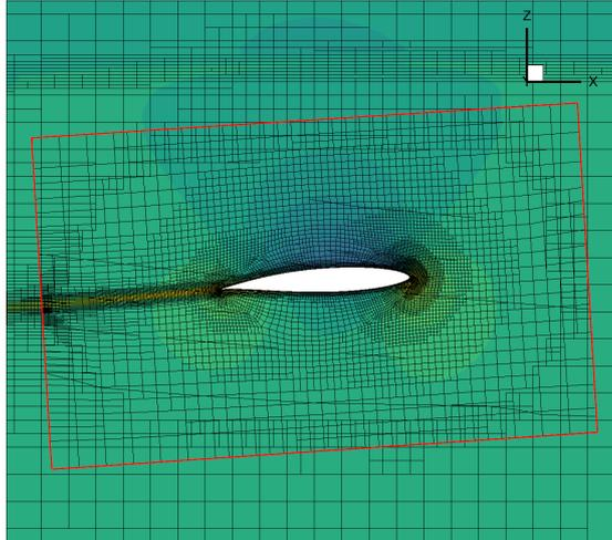
Figure 5: Cut through an overset domain around a hydrofoil, with matched refinement in the background and overset domains. The axial velocity is shown in colour.
