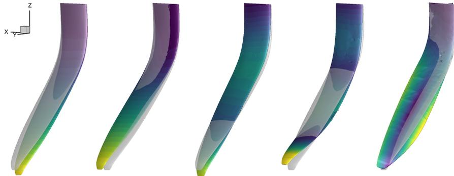
Figure 23: Eigenmodes  $\phi_1 - \phi_5$  (left to right) of the Nacra 17 foil. The colours indicate the magnitude of the deformation; the undeformed shape is shown in grey. The eigenfrequencies  $f_1 - f_5$  are 12.98, 31.23, 59.95, 141.11, and 217.95Hz.
