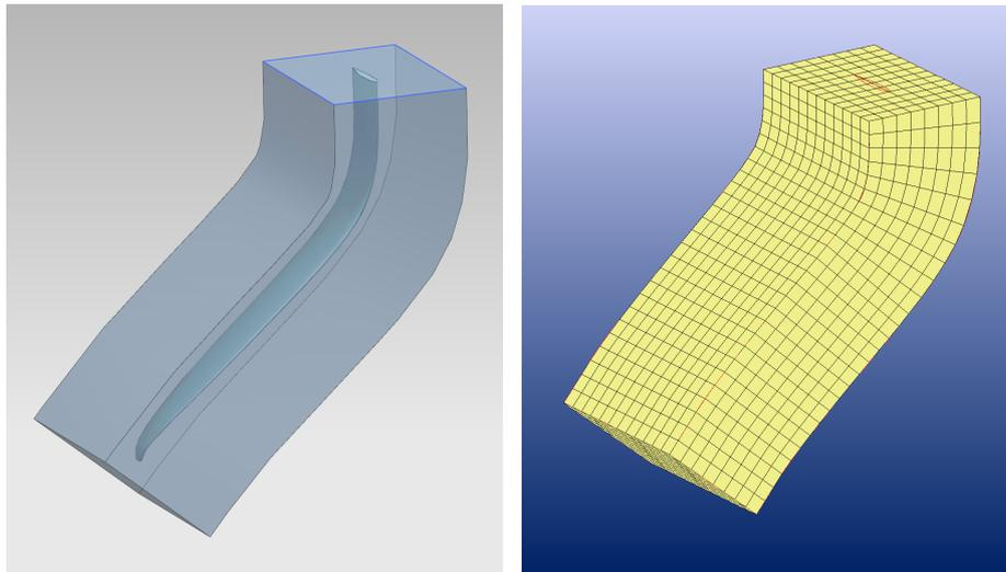
(a) The foil-shaped domain (b) Initial mesh created in this domain
