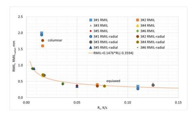
**Fig. 12.** Steady-state values of RMIL and RMIL radial as a function of RL for the flight samples, determined from radial and longitudinal cross-sections. Also added a fitted curve for the equiaxed values of RMIL and RMIL radial.
