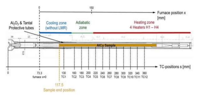
**Fig. 1.** Schematic setup of the SCA inserted in the SQF of the MSL on-board the ISS. The SCA contains the Al–Cu alloy inserted as a cylinder of 8 mm diameter and 276 mm length. The SQF is shown schematically at its initial position with respect to the SCA. It moves to the right during the solidification experiment. The positions of the 12 thermocouples TC1 to TC12, are distributed evenly along the sample.
