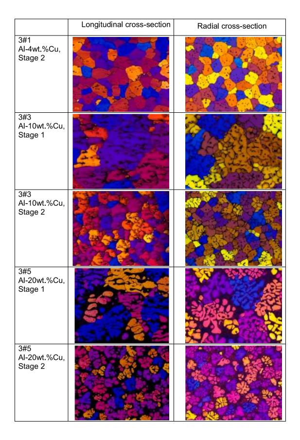
Fig. 11. Selected representative micrographs of the electrolytically etched cross-sections (height x width =  $2.10 \text{ mm} \times 2.65 \text{ mm}$ ) of flight samples CETSOL 3#1, 3#3 and 3#5 showing
