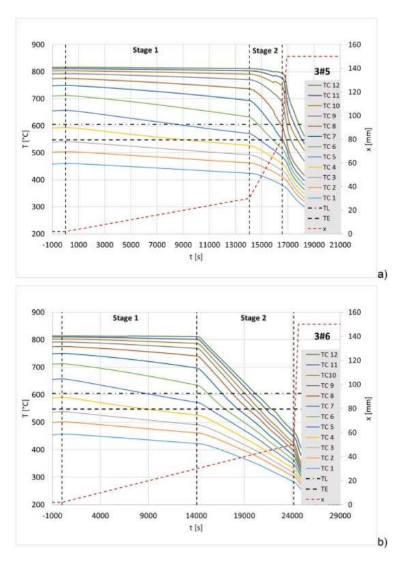
**Fig. 4.** Recorded temperature curves at thermocouple positions TC1 to TC12 and furnace position x (Fig. 1) for a) sample 3#5 and b) sample 3#6. The solidification stage 1 begins at t=0 s. Liquidus and eutectic isotherms of the Al-20wt.%Cu alloy (TL = 605°C and TE= 548°C [44]) are indicated with black horizontal dashed lines. The solidification stages are marked by dashed vertical lines. The red dashed line corresponds to the position of the furnace.
