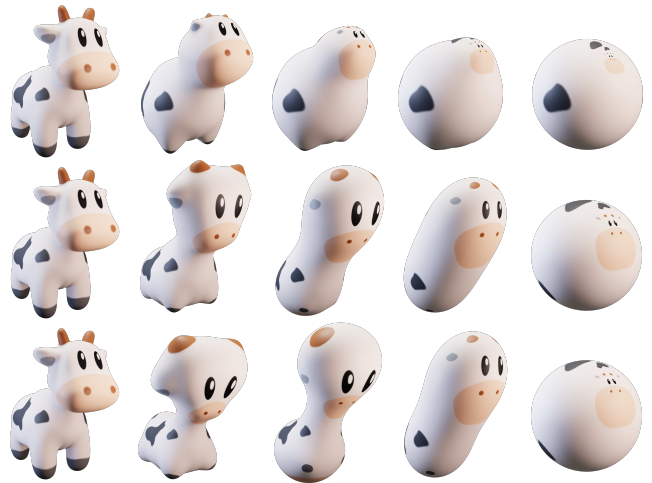
Fig. 1. Minimizing bending energy in Eq. (1) on spot for p equal to 1 (top, Willmore flow), 2 (middle) and 3 (bottom).
