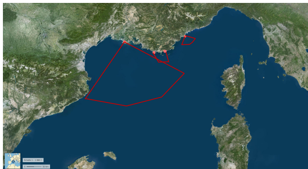
Fig. 1. Location of the 3 HFSWR networks on the French Mediterranean frontside together with their approximate spatial coverage. The ONERA operates a single station in Aigues-Mortes as of 2024; the MIO operates 2 WERA® stations in the region of Toulon and onde SeaSonde® station in Nice.
