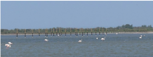
Fig. 2. Two of the four RX sub-arrays of the ROS NG in the salt pond of Aigues-Mortes.
