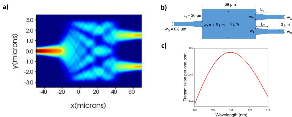
Fig. 4. (a) Simulated E field profile for MMI at 405 nm, (b) Dimensions of the simulated MMI ( $w_G$  is the waveguide width,  $w_T$  is the taper width and  $L_T$  is the taper length), (c) Transmission as a function of the wavelength of the SiON-based multimode interferometer designed for a 405-nm-wavelength propagation
