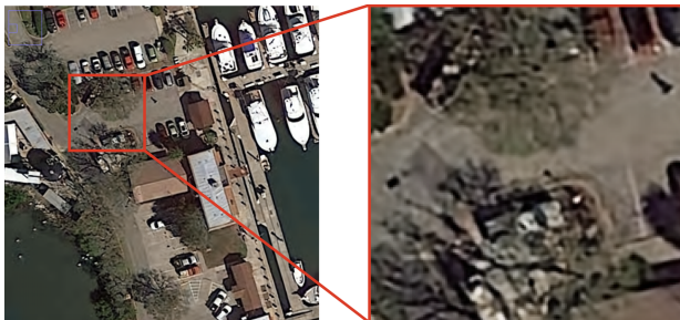
Fig. (12) Visual example of decompressed image and specific zoom area presented in [25]. This image was compressed at 0.096 bps (0.28 bpp) obtaining a reconstruction quality of 29.65 dB PSNR.
