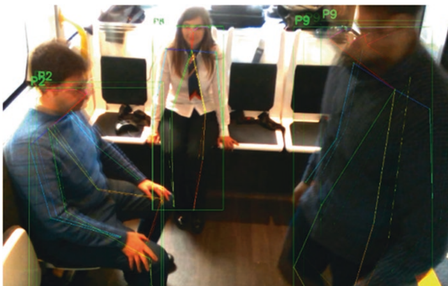
Fig. 5.2 Skeleton matching across two subsequent frames (blended) (Tsiktiris et al., 2020). Notice that the passenger ID, highlighted in green at the left of each bounding box, is the same across the frames
