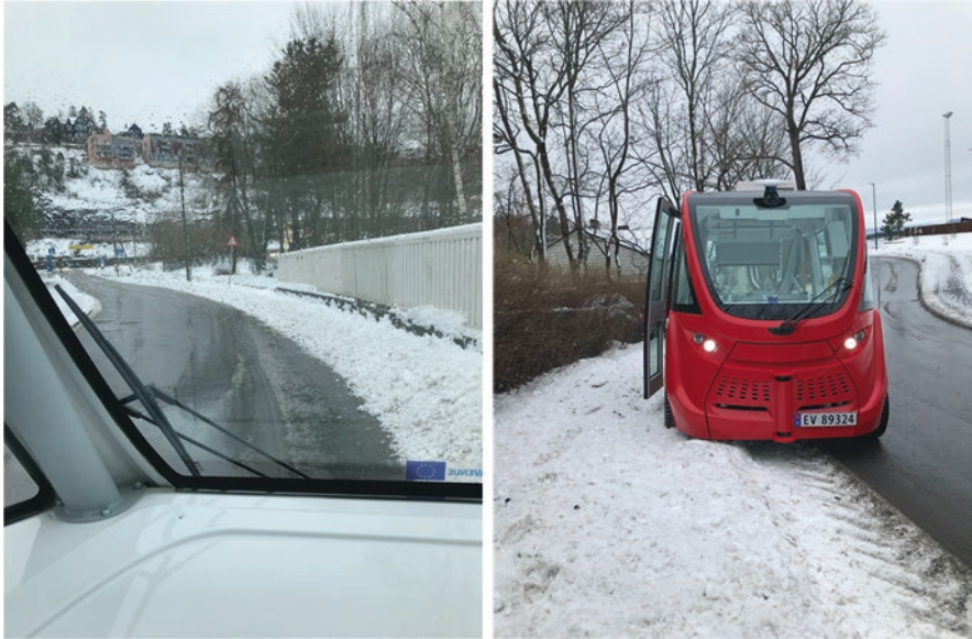
Fig. 2.14 Photos showing snow and snow banks in and close to the vehicle's trajectories on the route at Ormøya
