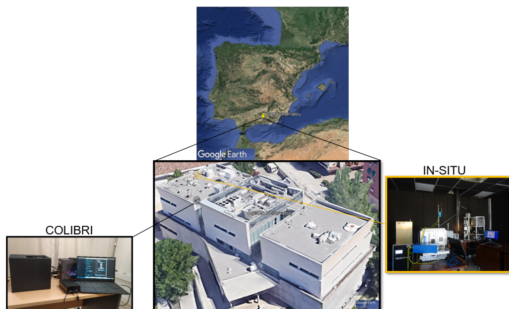
Figure 1. Deployment of the instruments at the AGORA Observatory, Granada (Spain), during the LiLOW campaign. The lidar and the in situ station are operated from the same buildings with a spatial separation between the in situ inlet and lidar output window of <10 m.
