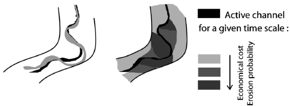
Figure 5. Schematic of the erodible river corridor concept. Left: illustration of historical changes in meanders, along with the boundaries of the erodible corridor. Right: illustrative example of assessment of the erosion hazard and risk within this erodible corridor (Source Piégay et al. 2005)
