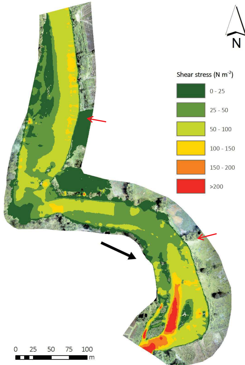
Figure 27. Shear stresses estimates from the 2D model at bankfull discharge ( Q = 75 \text{ m}^3 \text{ s}^{-1} ) for the lower reach.
