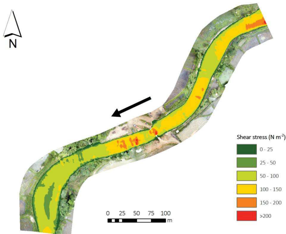
Figure 26. Shear stresses estimates from the 2D model at bankfull discharge ( Q = 75 \text{ m}^3 \text{ s}^{-1} ) for the middle reach.
