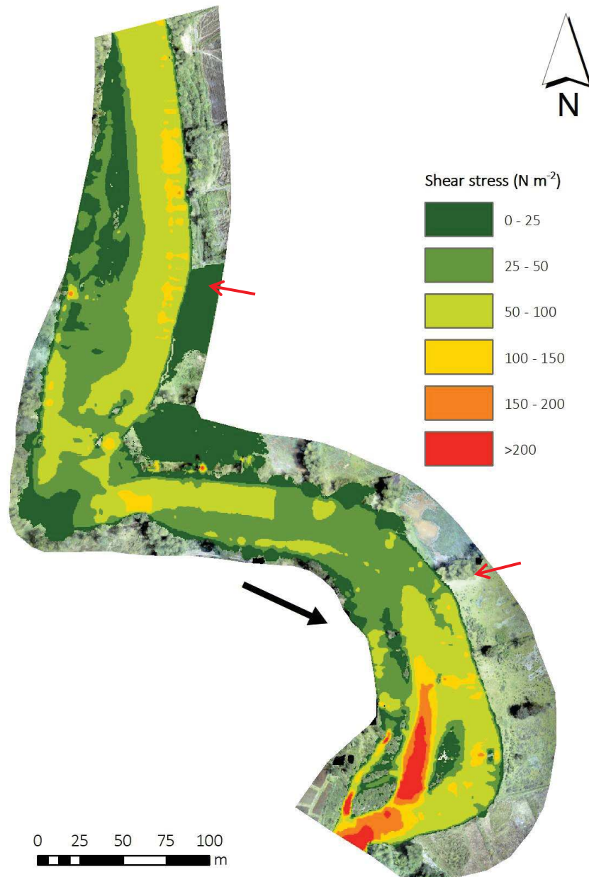
Figure 27. Shear stresses estimates from the 2D model at bankfull discharge ( Q = 75\ m^3\ s^{-1} ) for the lower reach.
