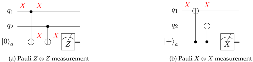
Fig. 10: Propagation of initialization errors through Pauli Z \otimes Z and X \otimes X measurement.
