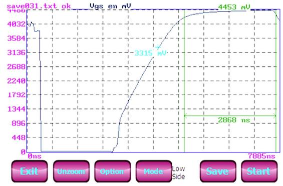
Fig. 7. Controller interface, visualisation of the health indicators on the extracted  $V_{GS}$  waveform (each indicator arises from dedicated derivative criteria). Here,  $V_{KN}=3315\text{mV}$ ,  $V_P=4453\text{mV}$ , and  $\Delta t_p=2868\text{ns}$ .
