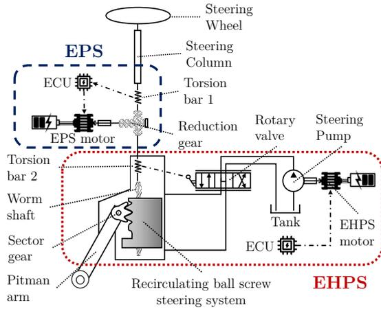
Figure 1: Simplified model of the Hybrid EHPS system.
