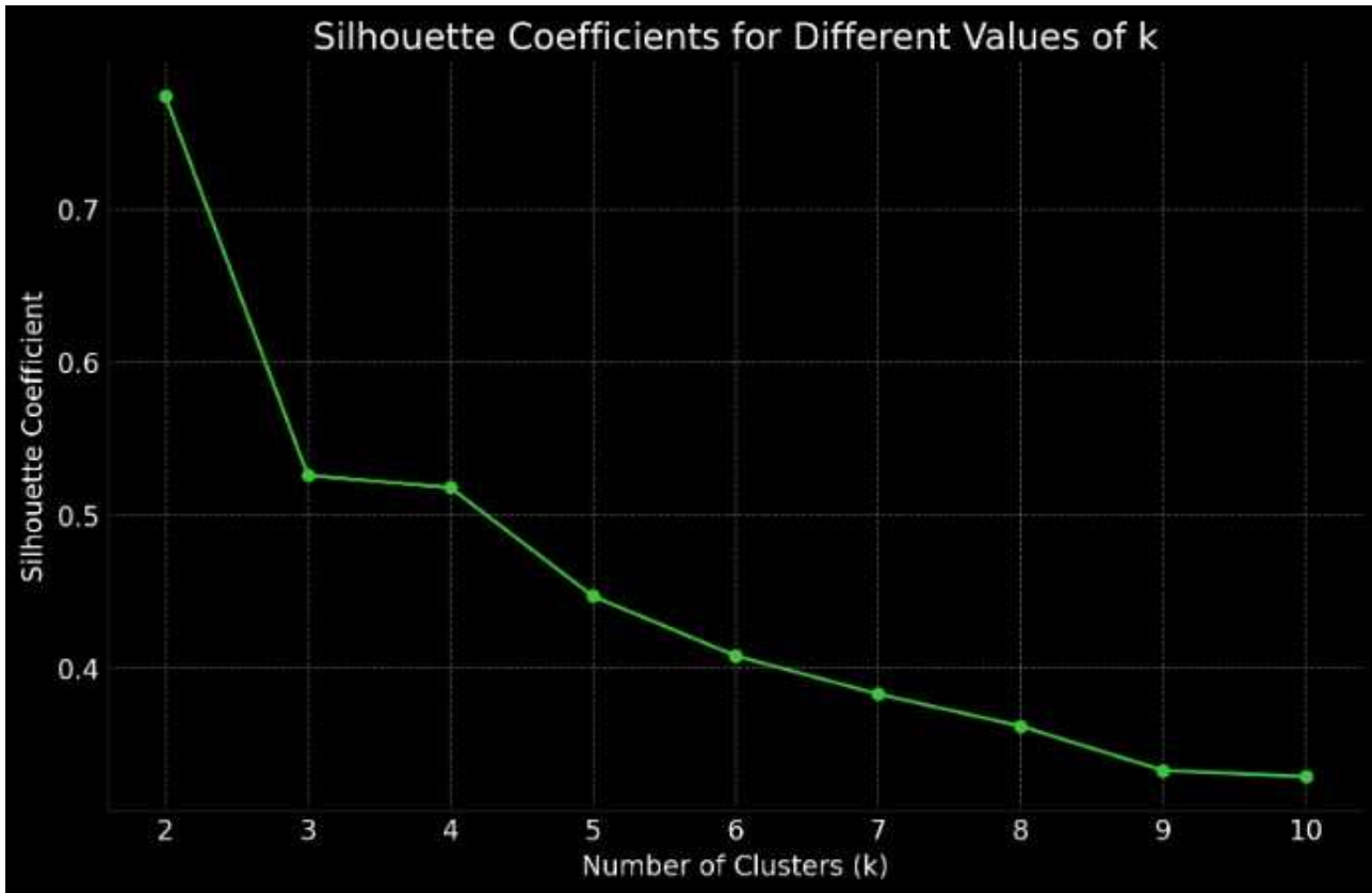
Figure 4. Here's the graph depicting the Silhouette Coefficients for different values of k from 2 to 10. The plot clearly shows that the highest coefficient is for k=2 , suggesting it as the most distinct clustering solution. As k increases, the Silhouette Coefficient generally decreases, indicating less optimal clustering.
