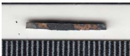
Figure 15. Photograph of the MEA/HfC alloy sample after the creep test
