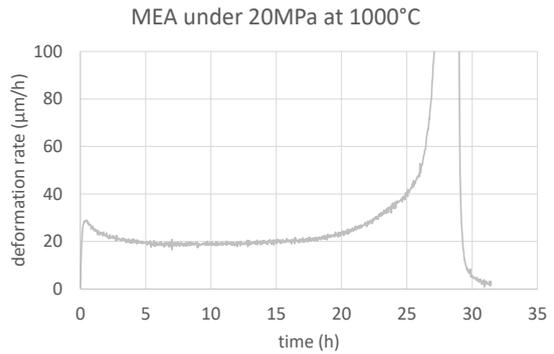
Figure 8. Central point displacement rate versus time for the MEA alloy
