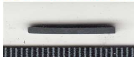
Figure 12. Photograph of the MEA/TaC alloy sample after the creep test
