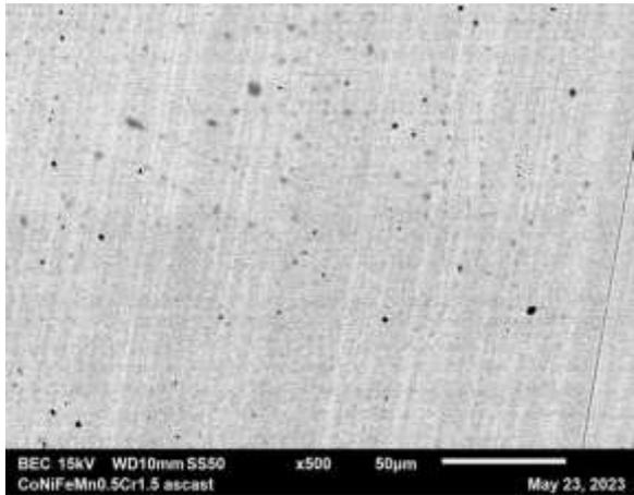
Figure 1. Back Scattered Electrons image of the microstructure of the MEA alloy (CoNiFeMn<sub>0.5</sub>Cr<sub>1.5</sub>)
