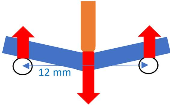
Figure 4. The principle of using the creep test
