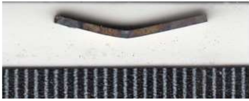
Figure 9. Photograph of the MEA alloy sample after the creep test
