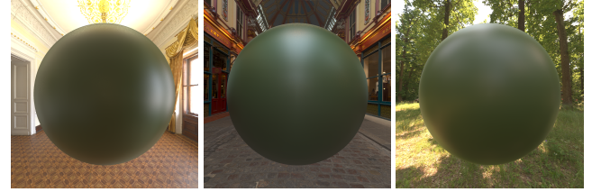
Figure 3: Results obtained in a rendering engine using the BRDF measured from a green paint sample using setup shown in Fig. 1 after interpolating data from sparse measurements for different environments.
