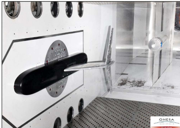
Figure 2-1: 1/8-scale flutter T-tail model wall mounted in the ONERA's S2MA transonic pressurized wind tunnel.
