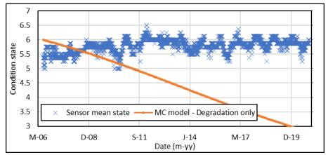
Fig. 2. MC model considering deterioration only.
