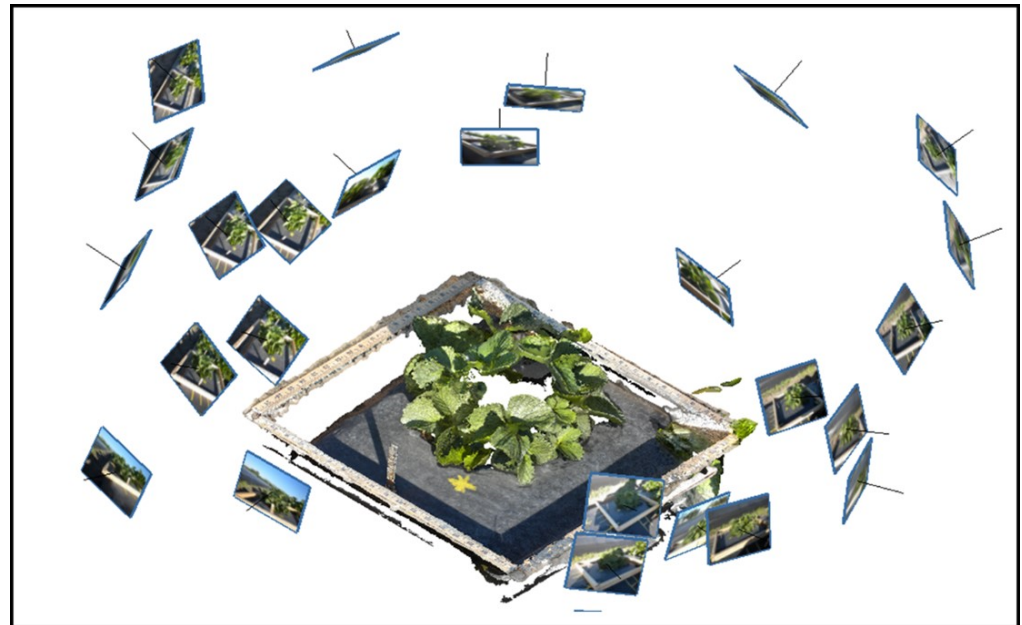
Figure 2. High-resolution, close-range image locations and orientations.
