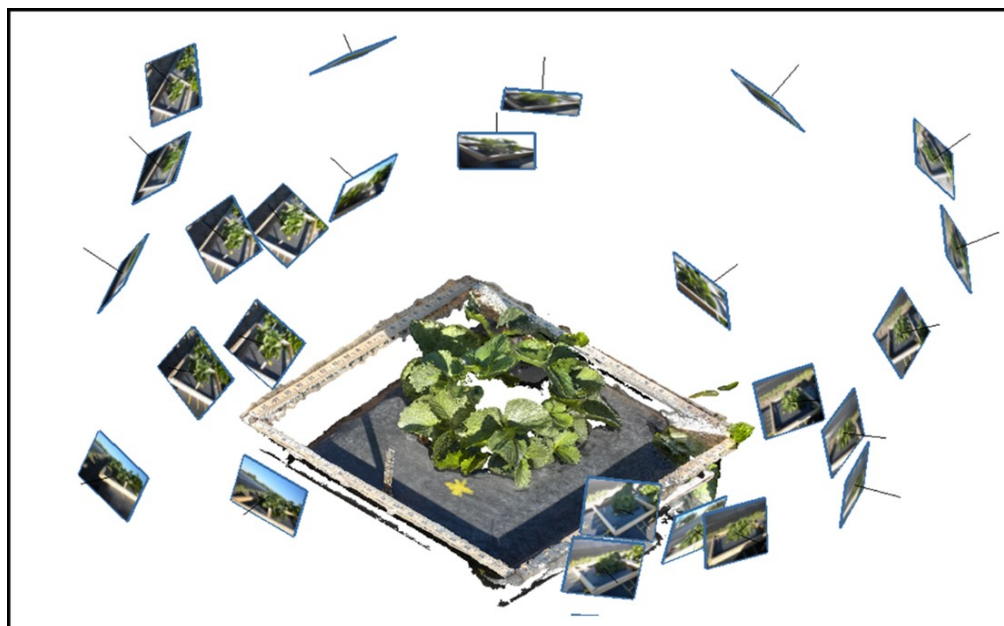
Figure 2. High-resolution, close-range image locations and orientations.
