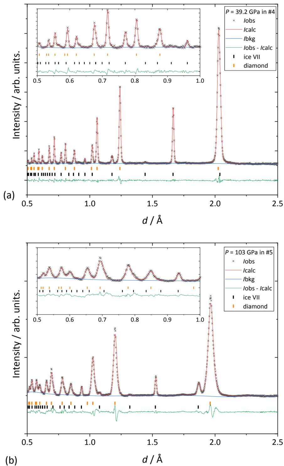
Figure 2. **Results of Rietveld refinements of neutron diffraction patterns for  $D_2O$  ice.** (a) at 39.2 GPa in run #4 and (b) at 101 GPa in run #5. *I*obs, *I*calc and *I*bkg means observed, calculated and background intensities, respectively.
