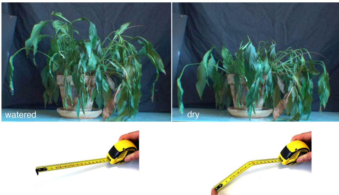
Figure 1. Spathiphyllum plant well watered (top left), and suffering a week without watering (top right). Metallic measuring tape undergoing a buckling instability (bottom line).
