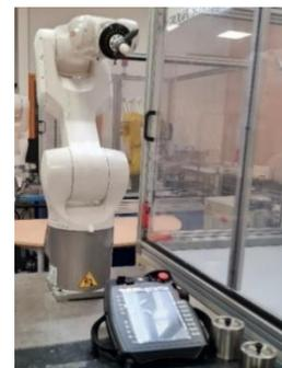
Figure 2. Robot industriel Kuka KR10
