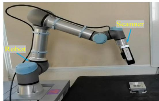
Figure 2 - Robot platform
