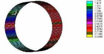
Fig. 8. Y^+ at the cylinder boundary for Re=10000
