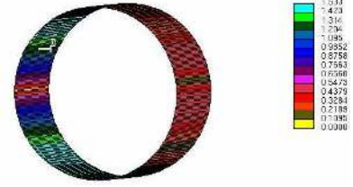
Fig. 8. Y^+ at the cylinder boundary for Re=10000
