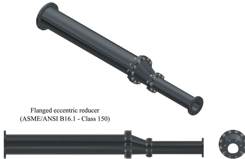
Figure 2. Assembly for the considered flanged eccentric reducer (ASME/ANSI B16.1 – Class 125).
