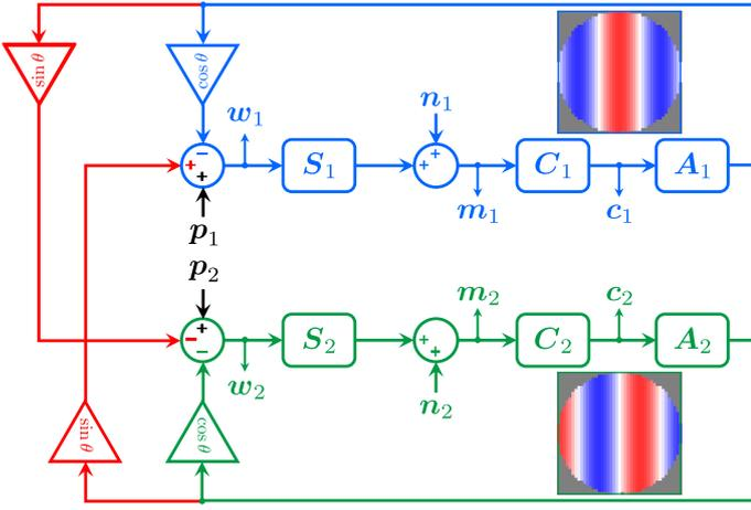
**Fig. 5.** Block diagram of the temporal coupling (in red) of the symmetric (cosine, in blue) and anti-symmetric (sine, in green) parts of a given spatial frequency  $\mathbf{k} = (2/3D, 0)$  through the AO loop.
