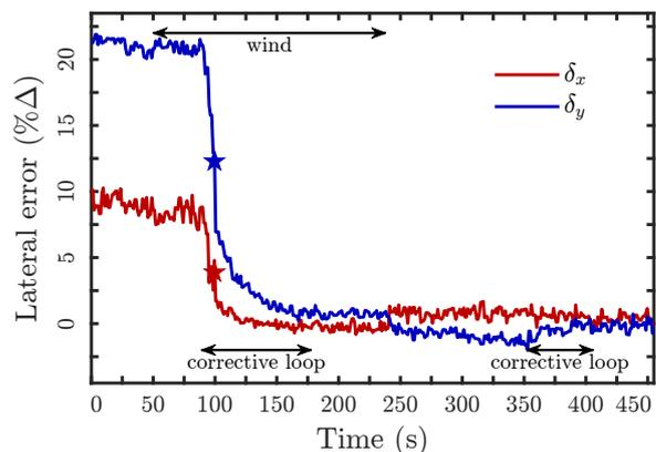
**Fig. 12.** Convergence of the lateral error corrective loop with the closed loop estimator. Double arrows indicate when the phase plate and the corrective loop are active. The stars indicate the iteration at which Figs. 11d,e are displayed.
