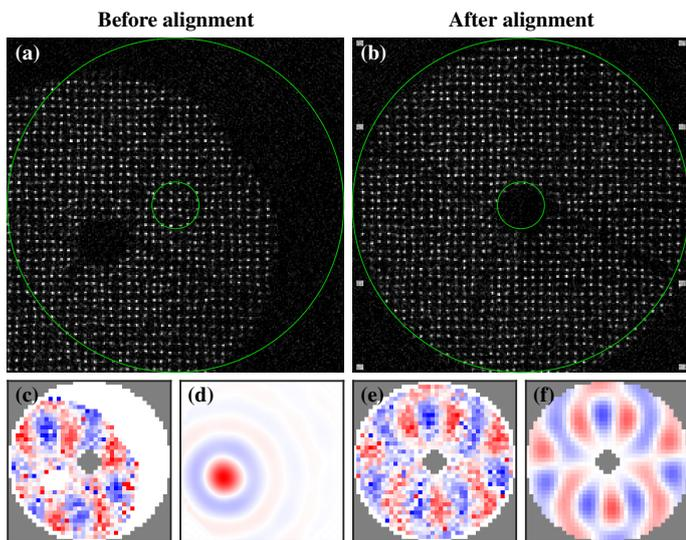
**Fig. 3.** Example in the GPAO bench of the 2D modal estimator. Panels a,b: SH-WFS pixels before and after the alignment. Green circles: WFS pupil edges. Panel c,e,f:  $x$ -slopes of the modal IM for  $m^{\text{KL}} = 40$  before (Panel c) and after (Panel e) alignment and reference (Panel f). Panel d: over-sampled map of the coefficient  $\alpha$  before alignment.
